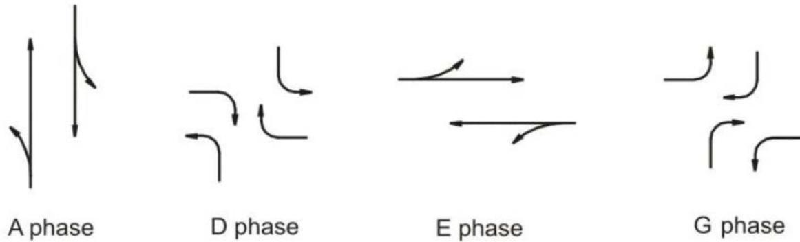
**Figure 9.3:** Example 'Double Diamond' Signal Phase Sequence
